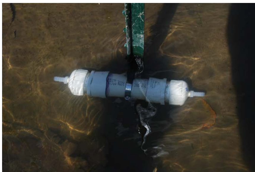
Figure 3.4 PSFM deployed about 4 inches below the water surface. Picture courtesy of Sarani Rangarajan.
