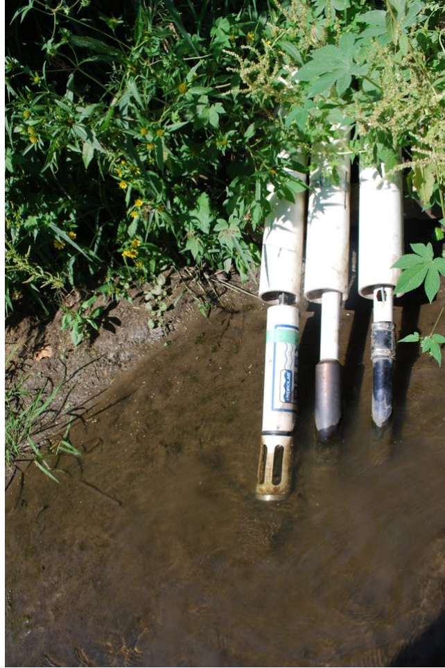
Figure 3.2 Water chemistry probe deployment by IIHR. Probes from left to right are pH, conductivity, temperature, and DO (Hydrolab), Nitrate as N (Hach Nitratax), and turbidity sensor (DTS-12 Forest Technology Systems). Picture courtesy of Sarani Rangarajan.
