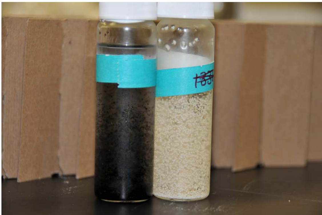
Figure 2.12 Extraction vials for alcohols and nitrate. The vial on the left is filled with Isobutyl Alcohol and alcohol dosed GAC. The vial on the right is filled with 2 M KCl and ion exchange resin.
